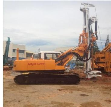
Figure 2: Micro piling machine
