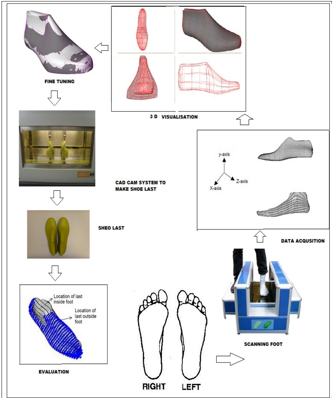
Figure 2. Flow diagram of custom shoe-last processing steps
