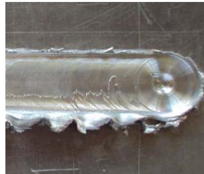
Fig. 5 : Macrostructure of first pass
