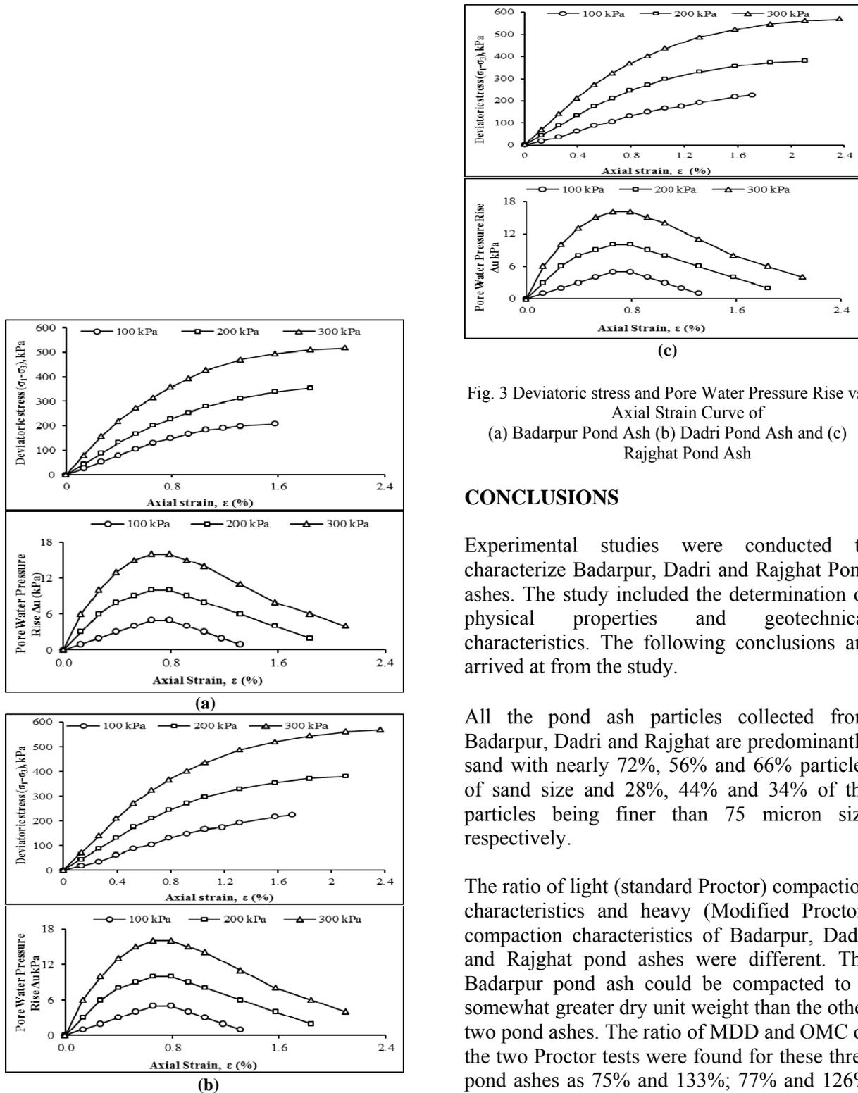
Fig. 3 Deviatoric stress and Pore Water Pressure Rise vs. Axial Strain Curve of (a) Badarpur Pond Ash (b) Dadri Pond Ash and (c) Rajghat Pond Ash
