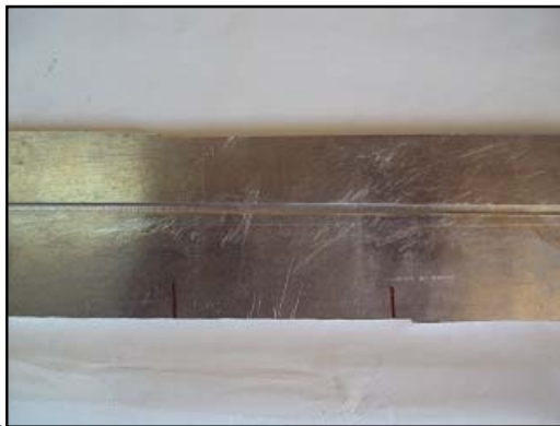
Fig.1 Picture of as-received Al alloy with groove
