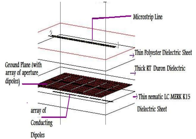
Fig 3: Sectioned Microstrip Layer
