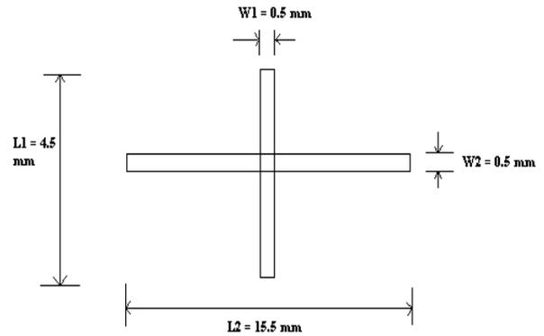
Fig 4: Schematic Microstrip structure with aperture and conducting dipoles sub-parameter's specifications
