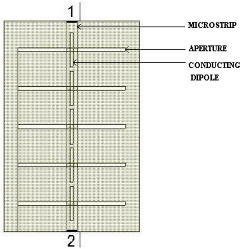
Fig 4: Schematic Microstrip structure with aperture and conducting dipoles
