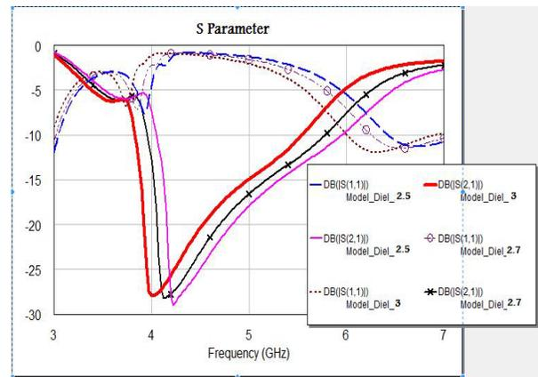
Fig. 8 Graph showing the comparing responses of the filter with dielectric permittivity 2.5, 2.7 and 3.0
