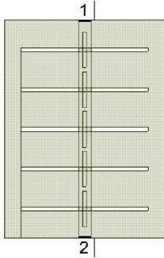
Fig 1: Schematic model Of EBG structure
