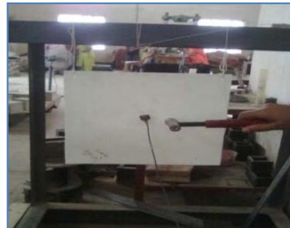
Fig. 3 : Iron Frame for making Free-Free B.C
