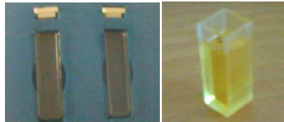
Fig. 1 : Cuvette holder and cuvette containing oil sample
