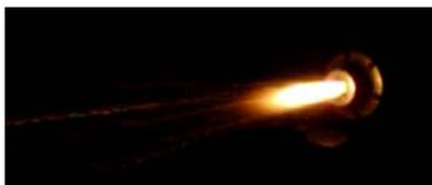
Figure.7 Schematic View of Solid Fuel (HTPB) Firing on Test Stand
