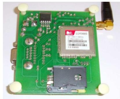
**Fig 2: GSM Modem**
