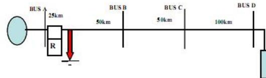
Figure 3: Single line diagram of simulated power network.
