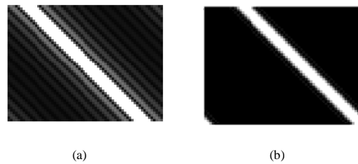
Figure 6: Matrices A ((a): optimal, (b): overlap-save using hamming window)
