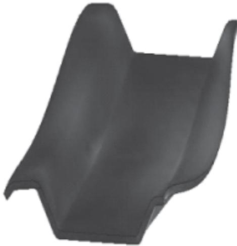
Figure 11. Failure mode from finite element simulation of experimental Set-up 3
