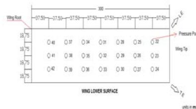
Figure 2. Wing Lower Surface; Pressure port Arrangements
