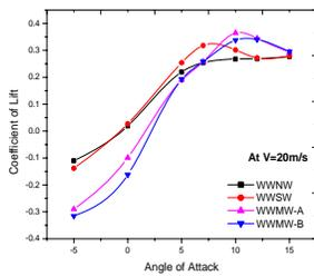
Figure 7. Comparison Curve; Coefficient of Lift ( $C_L$ ) vs Angle of Attack ( $\alpha$ ) in degree
