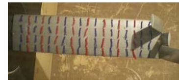
Figure 15. Tufts flow visualization for WMMW-A at  $\alpha = 10deg$
