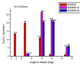
Figure 8. Angle of Attack ( $\alpha$ ) vs % of  $C_L$  increment over WWNW
