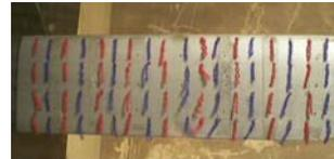
Figure 11. Tufts flow visualization for WWNW at  $\alpha = 5deg$
