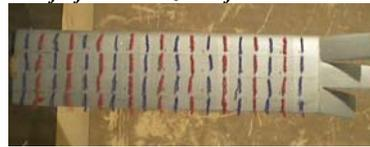
Figure 13. Tufts flow visualization for WMMW-B at  $\alpha = 5deg$
