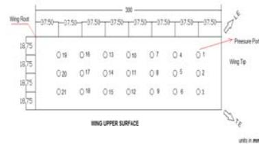
Figure 1. Wing Upper Surface; Pressure port Arrangements
