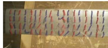
Figure 14. Tufts flow visualization for WWNW at  $\alpha = 10deg$
