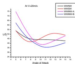
Figure 9. Comparison of  $L/D_i$  at various angles of attack
