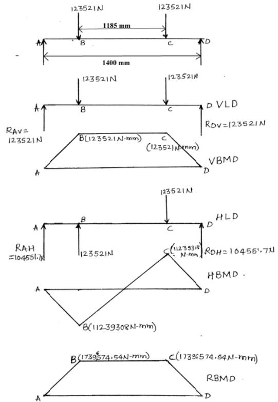
Figure 3.1: Bending moment Diagram
