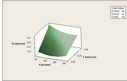
Fig. 2 Surface plots for Ra vs speed/feed
