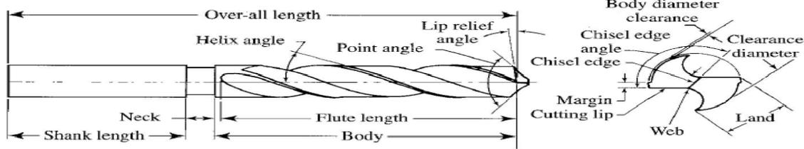
Fig.1: Configuration of a standard two-flute twist drill[14] and (b) an actual twist drill.
