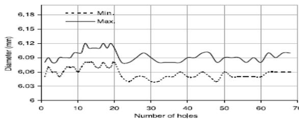
Fig. 3 Effect of the cutting speed on drilled holes after drilling with coated carbide drill B at a constant feed rate of 0.04 mm/rev 165 m/min.
