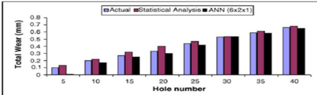
Graph 1. (Tool wear) diameter 8 mm, speed 9.04 m/min and feed 0.095 mm/rev.
