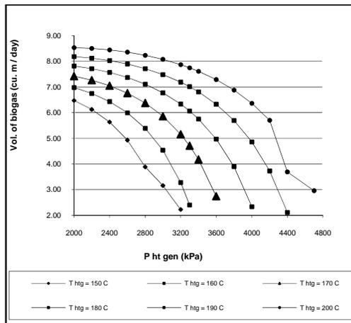
Fig. 4. Variation of pressure at high temperature Generator vs. Vol. of Biogas requirement
