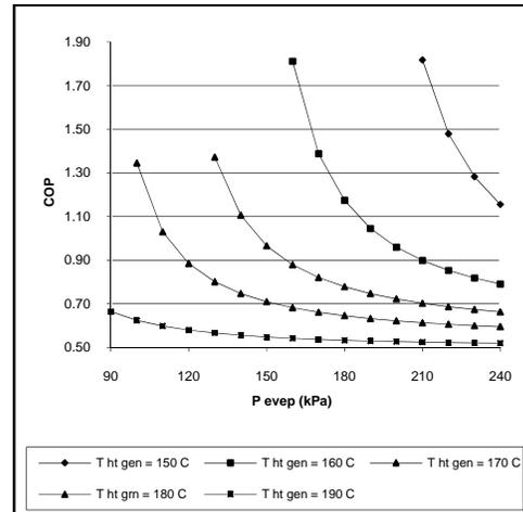
Fig. 6. COP vs. variation of pressure at evaporator
