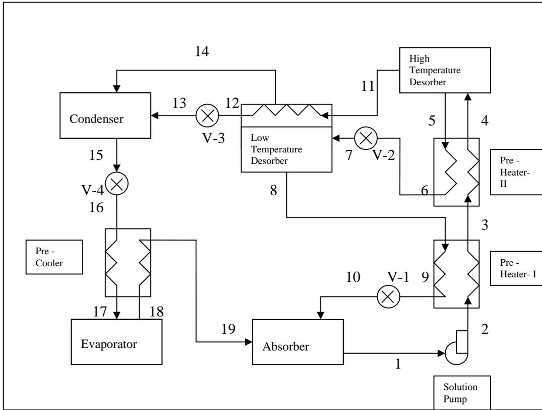
Fig.1: Double Effect GAX Vapour Absorption Refrigeration System
