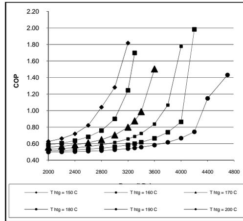
Fig. 2. COP vs. variation of pressure at high temperature Generator
