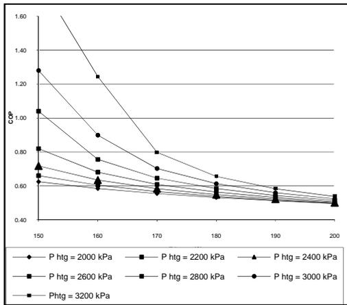
Fig. 3. COP vs. variation of temperature at high temperature Generator
