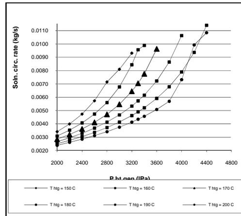
Fig. 5. Variation of pressure at high temperature Generator vs. Solution Circulation rate
