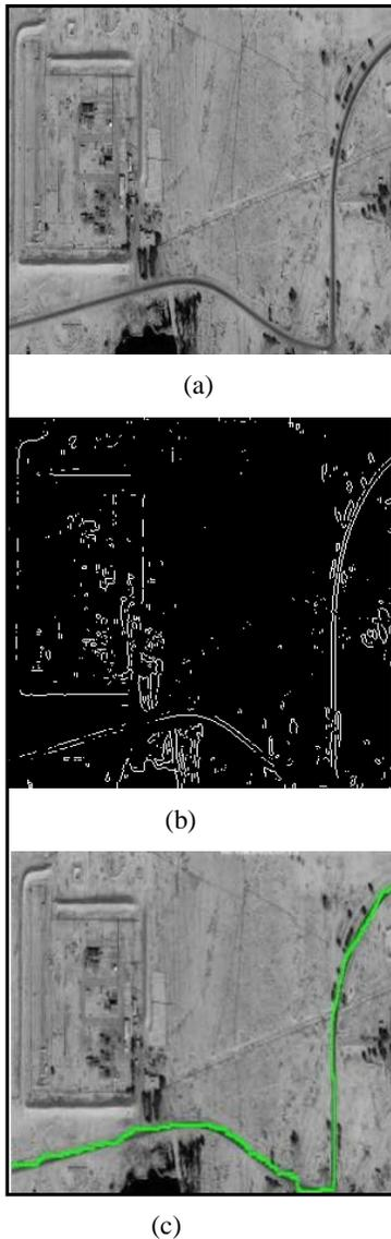
Figure.5 Road tracking results in an IKONOS image. (a)Reference profile extraction. (b)Edge detection using Sobel gradient mask (c) Road tracking by UKF
