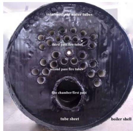
Fig. 2 front view of boiler shell
