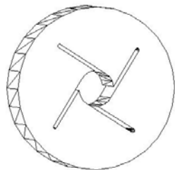
Fig. 2 nozzle-cup showing the flanges which provides the necessary pre-whirl to water flow.
