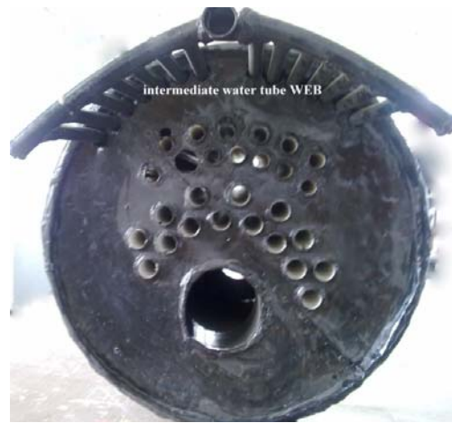
Fig. 1 back view of the boiler shell
