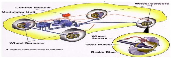
The EBCM then looks at the speed sensor signal from the affected wheel again. If that wheel is still decelerating, it opens the solenoid valve for that circuit. Once the affected wheel comes back up to speed, the EBCM returns the solenoid valves to their normal condition allowing fluid flow to the affected brake. Loss of hydraulic fluid in the brake master cylinder will disable the anti-lock system.
